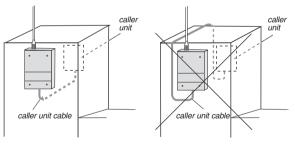
⑥ Also avoid placing the products close to metallic items (metal grilles, enclosures, metallic gates...) or sources of electromagnetic disturbance:
