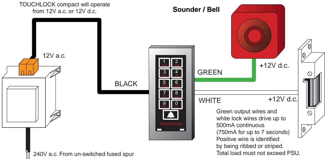
The green wires can be used to power a 12V dc door bell. There is a button on the keypad to activate the bell.
