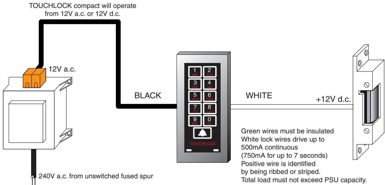
For 12V dc electric locks up to 500mA continuous power consumption or 750mA for up to 7 seconds. Fail closed and fail open locks can be used with TOUCHLOCK compact. The keypad can be configured easily (see **-TOUCHLOCK programming guide**).
