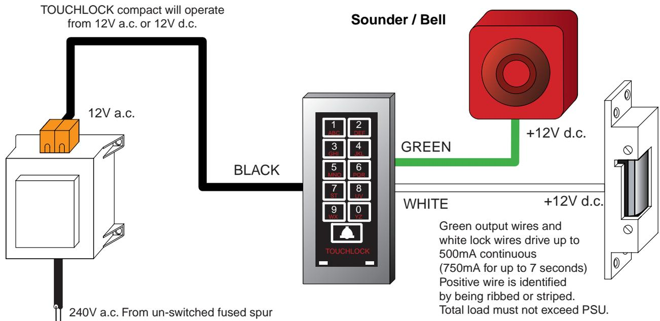
Duress codes can be programmed into the keypad. When a duress code is entered the lock output will activate for the door open time and the bell output will be activated for 30 seconds. The sounder and the lock current combined should not exceed the power supply rating.
