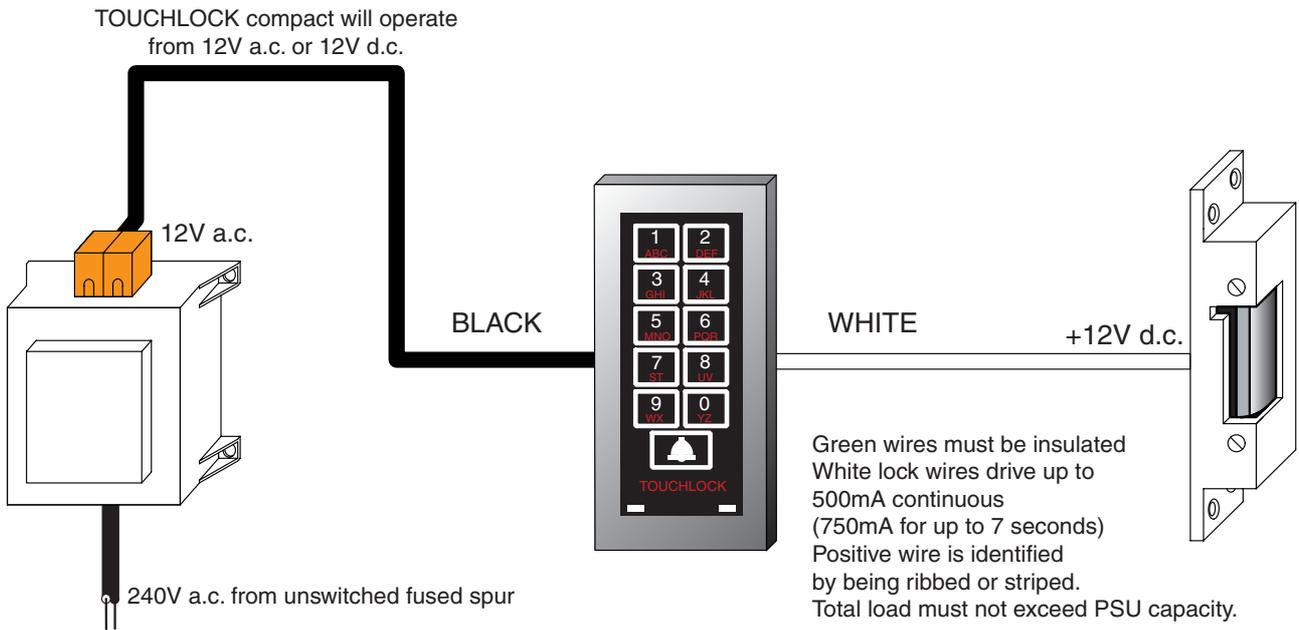
If the correct code is typed in, the release is activated and the door unlocks.
